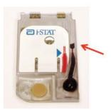
The sample well is overfilled, there is a bubble in the sample well.
