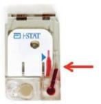
The sample well is insufficiently filled, and the sample does not reach the fill mark indicator.
