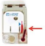
The sample well is insufficiently filled, and the sample does not reach the fill mark indicator.
