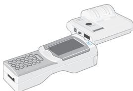
Before printing ensure that the printer is turned on. The printer is turned on and off using a switch on the left side of the printer. When the printer is on the Power LED will be green.
