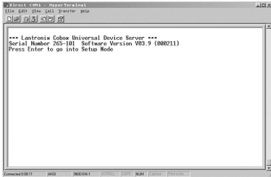
3. Press the Enter key immediately to enter the Setup Mode:
