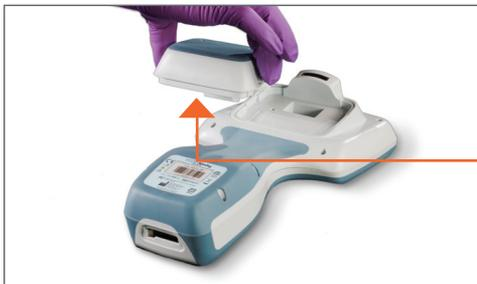
**BATTERY:** Rechargeable battery is the sole power source for the instrument.
