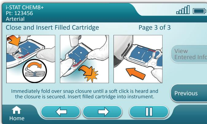
Below the Patient ID is the sample type selected from the previous screen or single sample type that is appropriate for the cartridge scanned. The action buttons at the bottom of the screen allow forward, backward and pause functionality.
