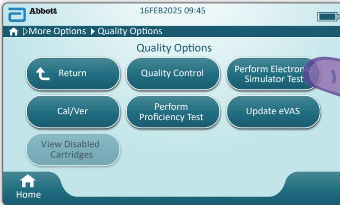
By carefully observing the text and graphic instruction, the user will be able to successfully complete an Electronic Simulator test. In the event that the test does not pass, follow the prompts on the screen.
