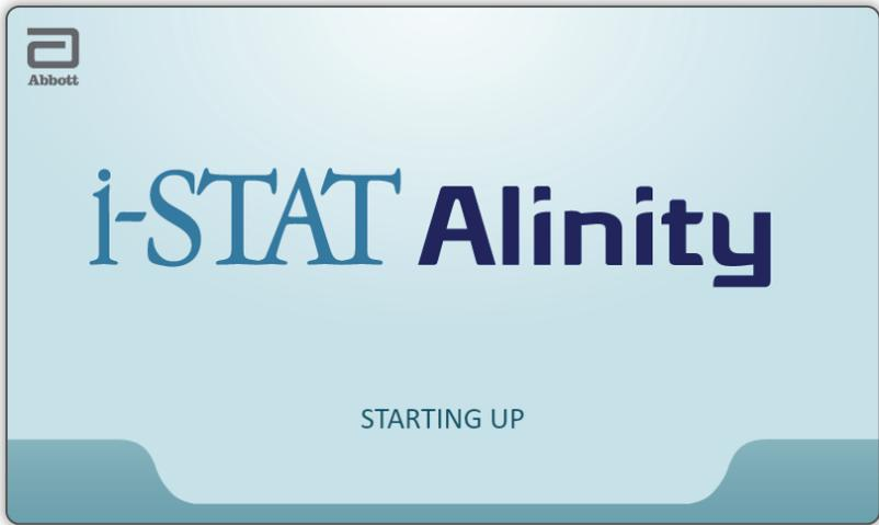
After the power button is pushed and the instrument starts the power-up sequence, the LED light will turn green, and i-STAT Alinity will appear briefly on the display screen. During the power-up sequence, the i-STAT Alinity instrument performs a series of self-checks.
